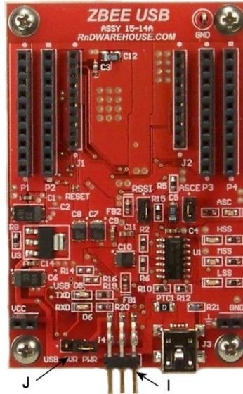
The AVR ISP Program Header J4 (**I**), requires a 6-Pin Ribbon cable for a 1-1 compatible connection to any AVR ISP Program Header. Looking into the connector **J4**, **Pin 1** is located in the lower left-hand corner.
