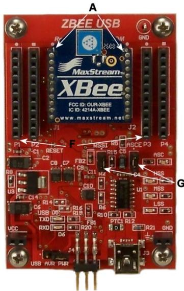
These additional support features are extended from the pins of the radio **(A)** to the P1 and P3 sockets **(F)**. This port extension allows the user to harness the full capability of the radio.
