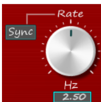
Figure 1: (Sync Off) set the LFO rate in Hertz from 0.10 to 10 Hz
