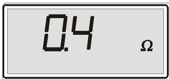
Fig. 9. Example of Rcon test result
