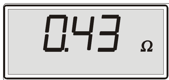
Fig. 8. Example of R_{\pm 200mA} test result
