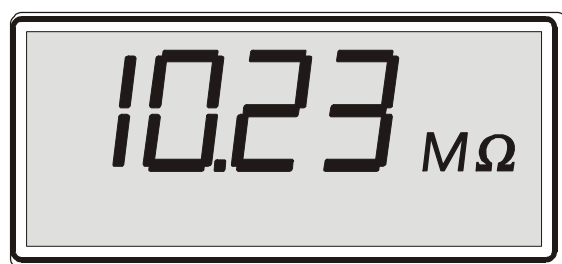
Fig. 6. Example of displayed insulation resistance result
