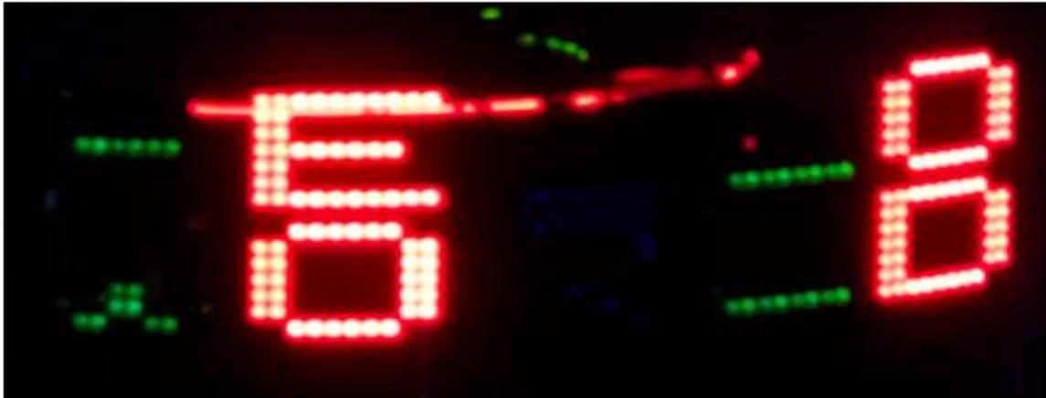
**Figure 7.5.7c: RGB Text Array displaying alternating color text.**
