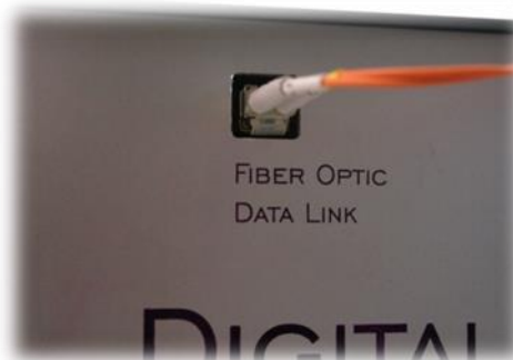
Figure 3-10 Fiber Optics input to EDT Card and DL
