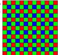
colored squares (typically well over a million), one for each pixel. This array of filters is called a Bayer filter array, after the Kodak engineer who invented it. The
