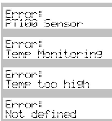
PT100 Sensor or cable defect.
