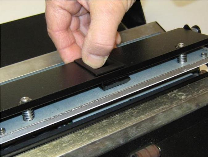
The Mini 8's print head is raised by pulling back on the sliding lock mechanism on the print head's top plate and rotating the print head assembly up as shown in the photo to the right.
