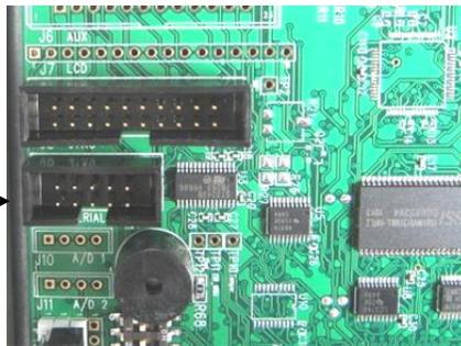
RS-232 Connector, J9 Pinout
