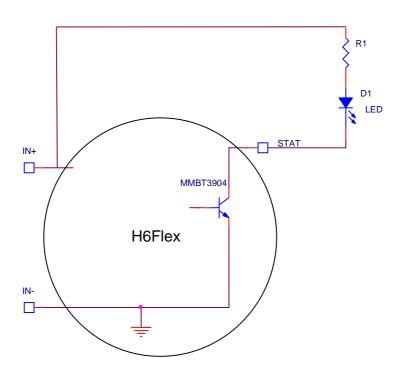
To calculate the value of R1 we need to know the input voltage, the Vf of the LED and the desired drive current to the LED.
