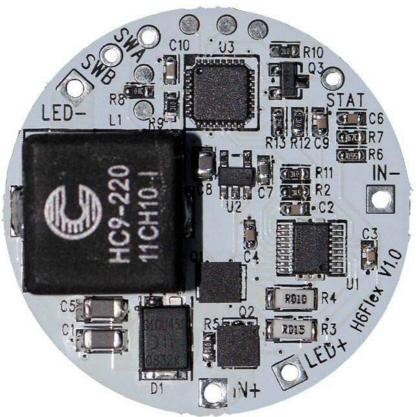
The picture shows the connections to H6Flex. The user provides DC power to the H6Flex (via battery, DC wallwart etc). H6Flex is reverse polarity protected with a low drop out FET (less than 50mV voltage drop across the FET).
