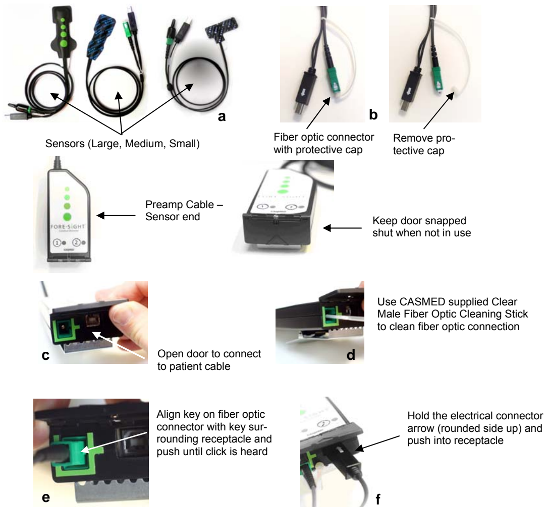
Figure 22: Connecting the Sensor to Preamp Cable
