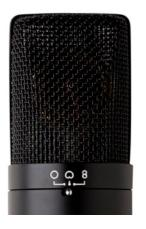
The three position polar pattern selector is a three-way switch found on the front side of the microphone. The selector allows the user to choose omnidirectional, cardioid or figure eight patterns.
