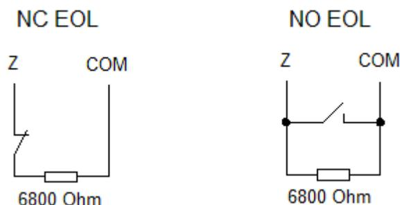
Loop resistance in the normal state must be 6,8kΩ
