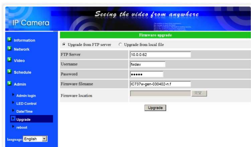
Figure 3-25: Firmware upgrade settings page
