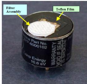
3. Remove the strip of Teflon tape that is attached to the Detector's Cell.
