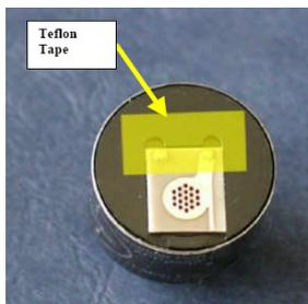
10. Place the sensor's Filter Assembly over detector's cell in the area where the holes are located. Make sure that filters are installed in correct order: clothlike filter on the bottom, filter with the backing – on the top.
