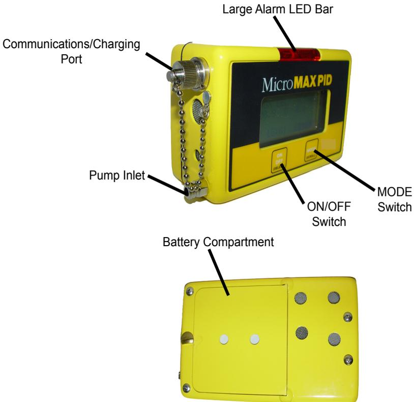
**Figure 2 - MicroMAX PID**
