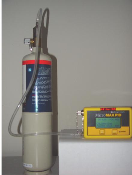
Figure 6 - Calibrating the MicroMAX PID
