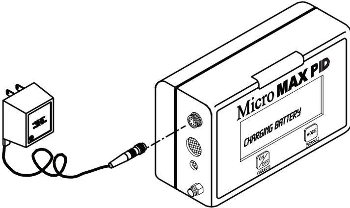
**Figure 1 - Charging the MicroMAX PID**
