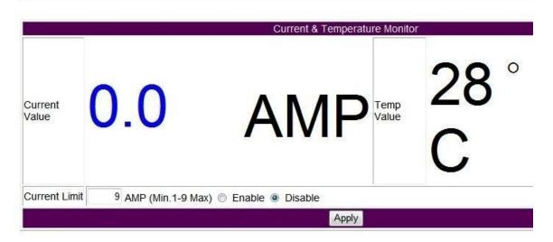
**Current Value:** Show the consume ampere of the device connected with **IPM-401S**. The tolerance of the current measurement is plus or minus at 10% degree.
