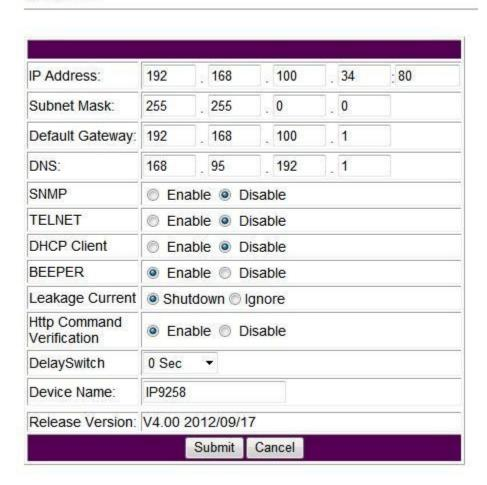
**IP Address:** IP Address of the **IPM-401S** device.
