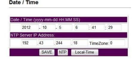
**NTP**: Network Time Protocol can be entered into the **IPM-401S**. Simply just enter the IP Address of the NTP Server and hit the NTP button to synchronize. Then press save .
