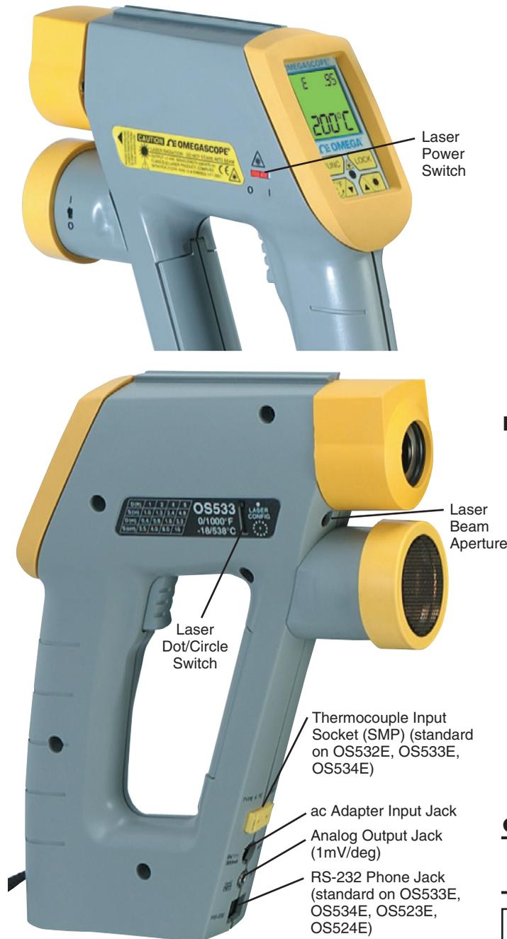
Figure 2. OS530E/OS520E Series Handheld Infrared Thermometer Various Views
