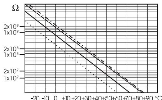
Since the resistance of the pH electrode is in the range of 50 – 200 Mohm, the current across the membrane is in the pico Ampere range. Large currents can disturb the calibration of the electrode for many hours.
