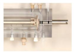
Insert the hex rod {1031573} and the driveshaft.
