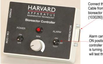
Connect the Communication Cable from the controller to the bioreactor motor housing {1030280}
