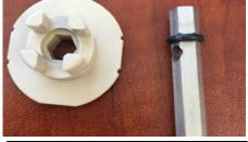
Place the small O-Ring {1030195} onto the end of the hex rod {1031573}.
