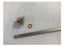
Place the O-Ring onto the shaft. A sterile pipette tip may be used to push the O-Ring into place.
