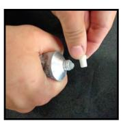
It is optional to apply **RTV Sealant** {1030566} to the threads of every port and fitting. A small amount, the size of a match head, should be applied to the thread to minimize the potential for leaks. Do not use too much RTV; a single drop will spread out and cover the entire area. Do not get sealant on the top of the fitting or the lids. When changing the fittings, use a Q-tip to clear debris while holding upside down to allow residue to fall out of chamber.
