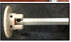
Push O-Ring in flush against the flex hole of the Support Inlet {1031588}
