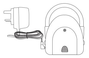
Power Supply : 230V 50Hz Output Voltage : 6V 200mA, I.2VA
