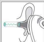
Braun ThermoScan measures the infrared heat generated by the eardrum and surrounding tissues. To help ensure accurate temperature measurements, the sensor itself is warmed to a temperature close to that of the human body. When the Braun ThermoScan is placed in the ear, it continuously monitors the infrared energy until a temperature equilibrium has been reached and an accurate measurement can be taken.
