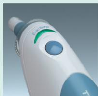
If you take the temperature of another person, the «ExacTemp» light can be of help. It flashes during the measuring process as long as the probe is correctly positioned, and lights up continuously when the thermometer detects that an accurate reading has been taken.
