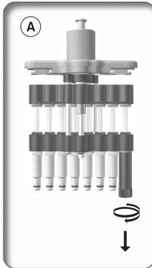
Push the mounting tool on and unscrew the single nose cone
