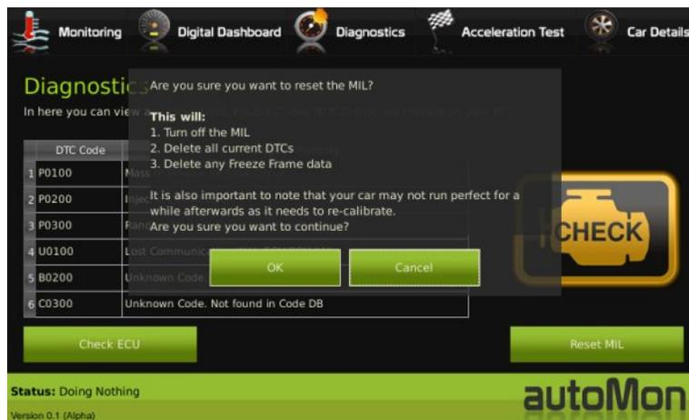
Figure 10 – Resetting the MIL and clearing DTCs
