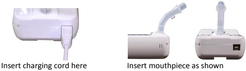
**NOTE:** The mouthpiece must be installed as shown here. The device will not accept a test if the mouthpiece is installed incorrectly. You are responsible for any missed tests due to the mouthpiece being installed incorrectly.
