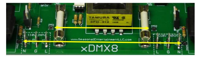
Power input connect can be made on any bank of input terminal tabs. It does not matter which side you choose.
