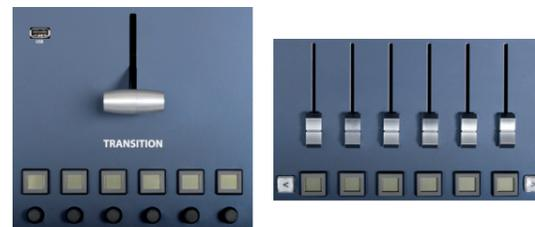
Below each fader you will find a screen button, you can use the left/right arrow to move this screen list. Each fader will take the screen which is written on the button.
