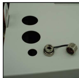
RJ-45 port on enclosure
