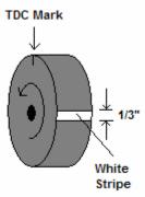
Once marked, turn the crank, as necessary, to allow access to the marked portion of the balancer. Paint a  $\frac{1}{3}$  –  $\frac{1}{3}$  wide white or silver mark on the balancer at the marked point, as shown above.
