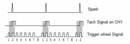
One can see that the measurement window is shifted by the width (or time duration) of the Trigger wheel pulse. Because in most cases that pulse width is fixed, the error translates to varying number of degrees depending on RPM.
