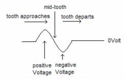
When the gear tooth approaches, the magnetic field strengthens and a positive voltage gets created. (by convention, the voltage direction is positive for an approaching tooth). The coil, by that convention, has a positive and a negative end.
