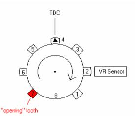
From this we know that the missing tooth (number 8) passes by the VR sensor at 90 degrees BTDC. The missing tooth is 180 degrees before TDC. The VR sensor is offset from that in counter-rotating direction by 90 degrees, so 180 - 90 = 90.
