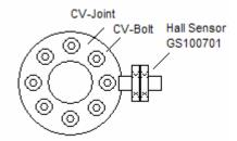
The hall sensor used in this case is a Cherry GS100701 with built-in magnet. It can be found at <u>www.digikey.com</u> as P/N CH398-ND.
