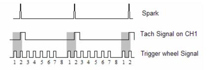
One can clearly see that the falling edge of the tach signal is outside the measurement window. If for example the tach signal contains the spark signal of all sparks of an 8 cylinder engine, the spark event of cyl. 8 instead of cyl 1 could fall into the measurement window and the measurements would be off.
