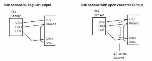
A Hall sensor with an open collector output needs a load resistor (example 4.7k Ohm between it's output and +5V.
