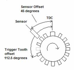
In this case the offset of the Trigger Tooth is 112.5 degrees (passes TDC in 112.5 deg after TDC). The sensor is mounted at 45 degrees after TDC (After TDC here is opposite to rotation direction). So the complete real offset from TDC is 67.5 (112.5 - 45) degrees after TDC.
