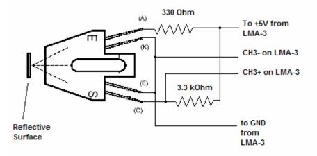
Paint the balancer or flywheel surface flat black so as to reflect minimal light.
