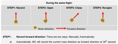
after you power on the multi-rotor. And LED will blink quickly if recording is successful.
