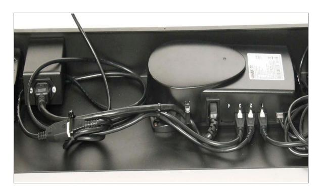
6. Place cover back on the base and secure with (5) screws.
