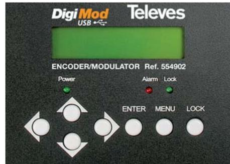
**LCD Display** – It presents the selected menu screen and the parameter settings. The backlight in the display is on when the power is applied.
