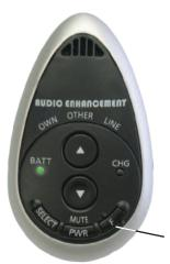
If your classroom is equipped with the **SAFE** System you can send an alert by pressing and holding the Function button on your microphone. Three Blue LEDs will illuminate on the face of the microphone and three Red LEDs will illuminate on the ceiling mounted dome sensor indicating that the ALERT signal has been sent.
