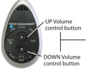
Press either the UP or DOWN arrow button to increase or decrease the level of the Teacher microphone. A blue LED over the "OWN" (for own microphone) will flash with each press.
