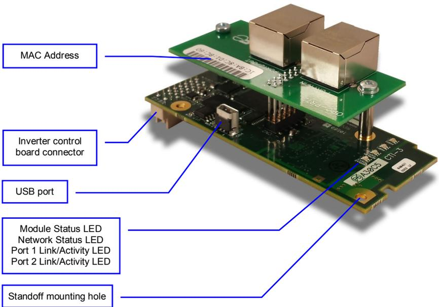
Figure 5: OPC-PRT2 Component Overview (Reverse View)
