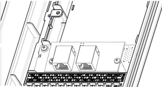
**Figure 8: Interface Card Mounting Completed**
