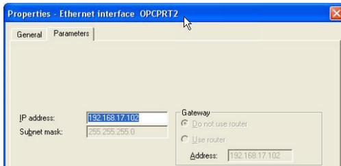
**Figure 48: Assign Unique Compatible IP Address**
