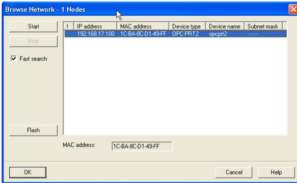
Figure 51: Discover PROFINET Devices on the Network
