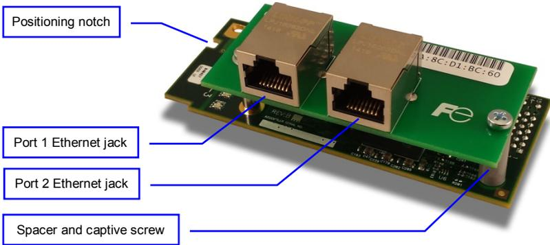
Figure 4: OPC-PRT2 Component Overview (Front View)
