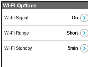
5. To disable the Wi-Fi signal in a restricted area, tap the > button next to Wi-Fi Signal.
