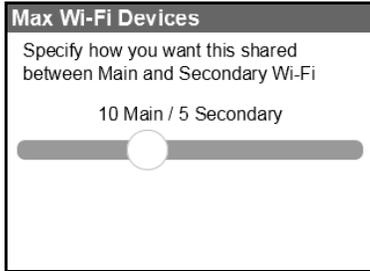
6. Slide the button to specify how you want the Wi-Fi devices to be shared between each Wi-Fi network.
