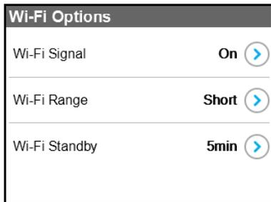
5. To disable the Wi-Fi signal when you are on a USB tether, tap the Wi-Fi Signal > button.
