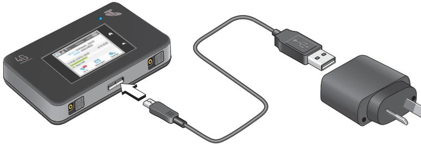
2. Plug the wall charger into a wall socket.
