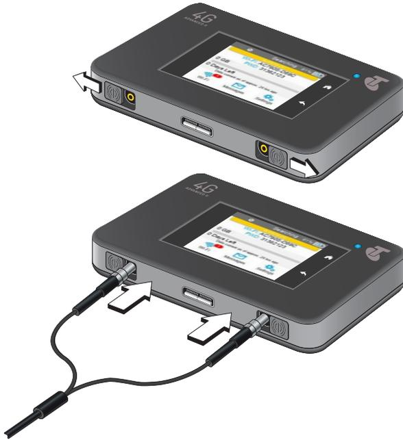
Figure 4. External antennas with TS-9 connectors
