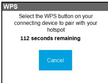
6. Within two minutes, press the **WPS key** on the wireless device you want to connect.
