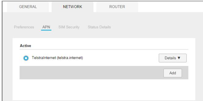
5. In the blank row, enter the name of the network service provider and the APN that you obtained from it.
