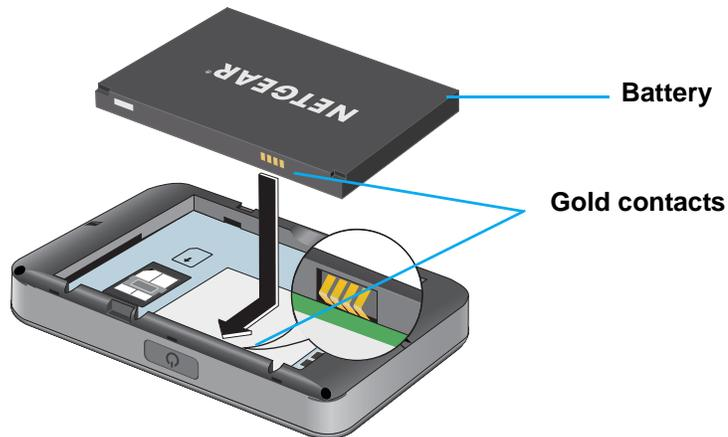
Ensure that the gold contacts on the battery line up with the gold contacts on the device.
