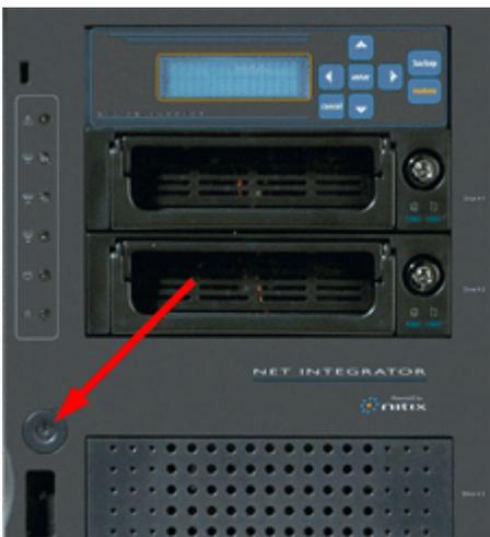
1. Press the Power button (located on the front of your Net Integrator).
