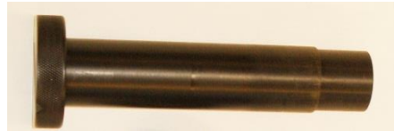
Figure 15: The sighting tool for 45° transducer holders.
