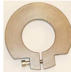
Figure 16: The stop washer for the sighting tool for the 42°/48° transducer holders.
