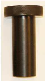
Figure 14: The sighting tool for the 42°/48° transducer holders
