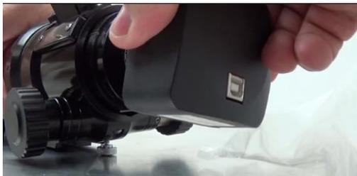
Insert the SkyRaider-DS (with C-Mount attached) into a 1.25" eyepiece adapter on your Telescope.
