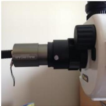
Insert the **SkyRaider-G** (with C-Mount attached) into a 1.25" eyepiece adapter on your Telescope.
