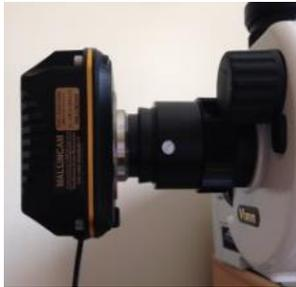
Insert the **SkyRaider-SLP** (with C-Mount attached) into a 1.25" eyepiece adapter on your Telescope.
