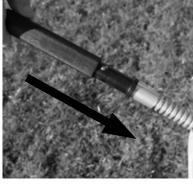
Slide the hinge lock tube over the hinge assembly
