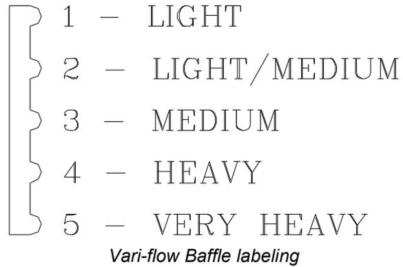
Each baffle is factory set base on the type of appliance under the hood.
