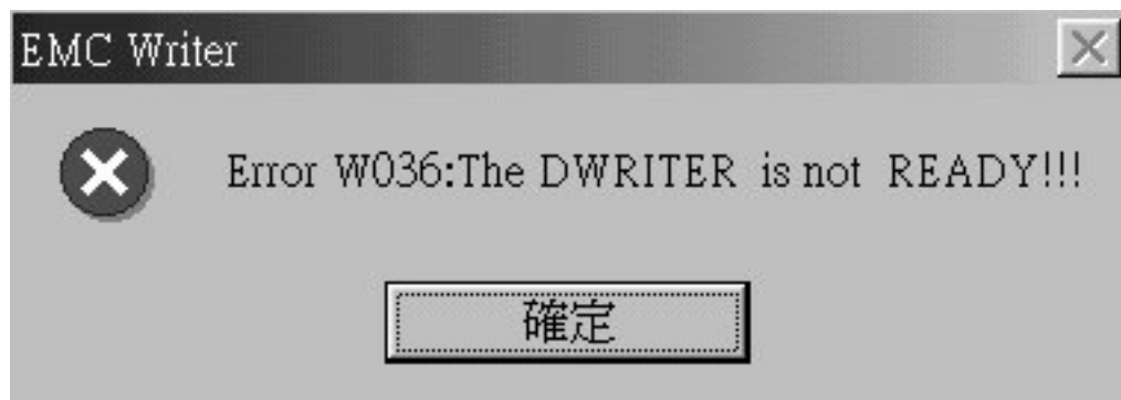
Fig.22. OTP not in socket or Short jump not connected
