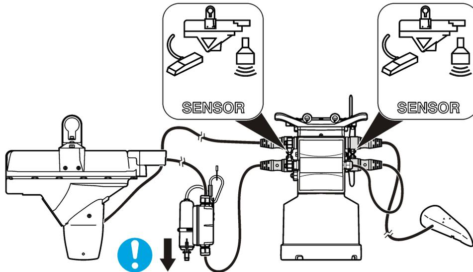
Figure 7 Attach a sensor to an external module
