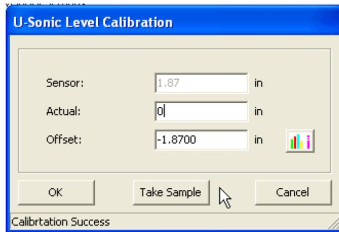
7. Click **TAKE SAMPLE**. The sensor measures the distance to the liquid surface and uses the sensor height information to calculate the liquid level. After approximately 45 seconds, the level measurement is shown.
