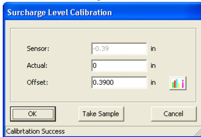
2. Click **TAKE SAMPLE**. The sensor measures the surcharge level. When complete, the value is shown in the Sensor field.
