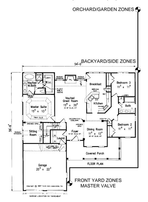
Based on the contractor's choices for valve locations, the simplest topology will be bus topology for the wire. Bury the wire along the water main line for the irrigation system. The water main line is the thick black line connecting the checker-patterned valve location markers. One IVC24-04 device will be located at each valve group. The total distance for the 24VAC bus wire will be around 150 feet.
