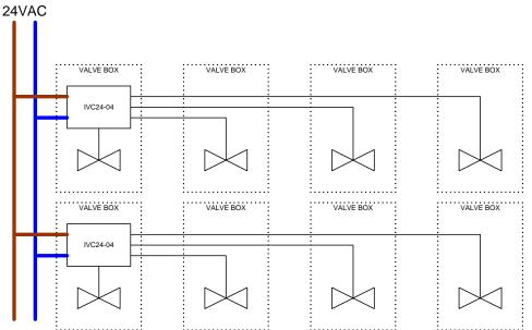
One advantage of the bus topology is a reduction in wiring costs compared to the star topology. Only two wires go out into the field to each valve group. Another advantage is the ease of adding more devices. Extending your system is as easy as tapping the nearest 24VAC bus wire, connecting an IVC24-04, and adding valves to the nearest water feed pipe.
