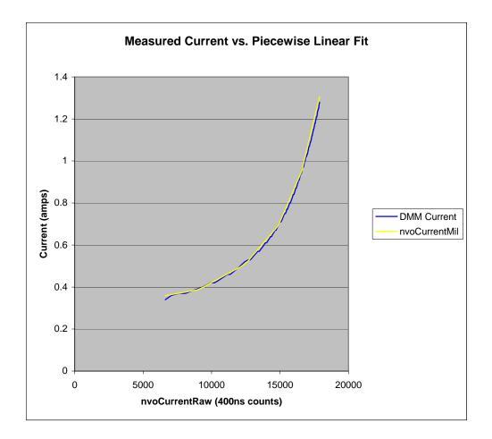
The X-axis is the raw network variable output "nvoCurrentRaw". The blue line is the current as measured by a DMM. The yellow line is the network variable output "nvoCurrentMil".
