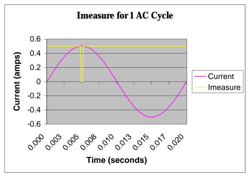
Imeasure is an active low digital signal shown in yellow and is scaled & overlaid on top of the current waveform. The peak of the current is around 0.5 amps and is just enough to trip the comparator.
