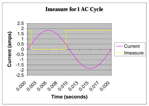
Two network variable outputs are provided from the current measurement circuit. The first, named "nvoCurrentRaw", is type SNVT\_count and is the duration in 400ns ticks that the signal Imeasure was low. For example, if the value of nvoCurrentRaw is 6500, the duration of the Imeasure pulse was:
