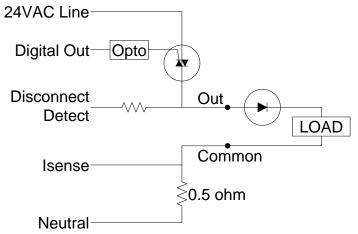
Connecting the diode with this orientation drives the load using the positive half cycle. This allows the load to sink the leakage current on the positive half cycle, which allows the disconnect detect circuit to sense the output is connected.
