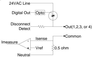
The output Imeasure will only trigger when the signal Isense is larger than the voltage reference Vref. Vref is set to approximately 0.25 volts with some hysteresis to reject noise. This means the minimum trip current will be:
