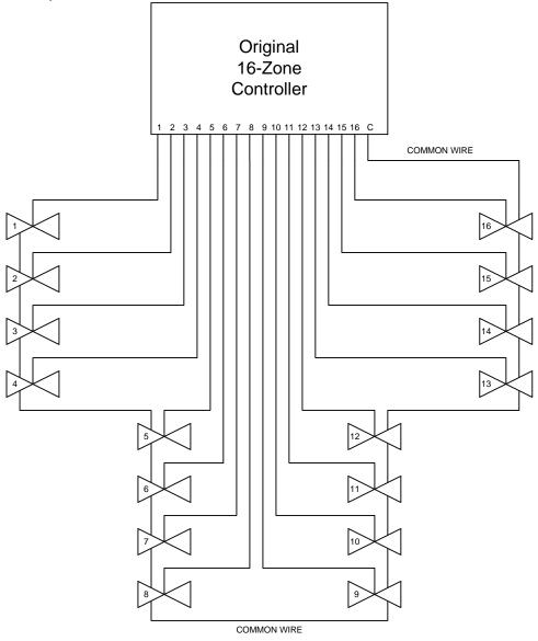
For the retrofit, every two wires would be connected together to bring 24VAC power to each IVC24-04 installed with each of the 4 valve groups like this:
