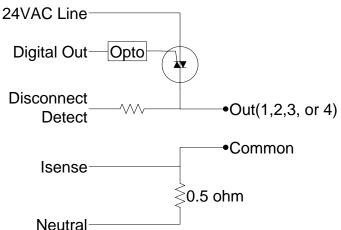
When the output is disconnected, a square wave (due to clamp diodes in the digital input of the microcontroller) is present on the digital logic side of the disconnect detect sense resistor. The microcontroller watches for this toggling input. If the input toggles for more than 6 cycles in a row, the output will be marked as disconnected. At 50Hz, therefore, it will take 6 AC line cycles, or 6 \* 20ms = 120ms to detect a disconnected output.
