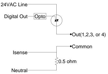
Note the 0.50hm current sense resistor is shared between all 4 output circuits. The 4 common wires are provided for wiring convenience. Connecting commons between different IVC24 devices will cause improper operation of the current sense circuit. See the section "Current Measurement" for more details.
