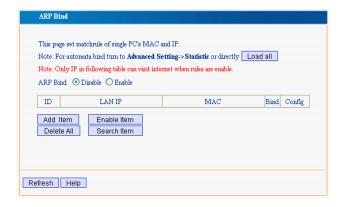
Notice: If you enable this function, there is no IP or MAC addresses in the table, then all the computers in the network are not able to connect to the network, only the IP and MAC addresses displaying in the table are entitled to have access to the network.
