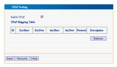
TEI480T+/TEI490T+/TEI4000+ supports the latest Universal Plug and Play (UPnP). It would be effective under OS Windows ME/ Windows XP or above (Remarks: The OS should be integrated, and installed with Directx 9.0 or above revision.), or under the applications which supports UPnP. For example, a computer under OS of Windows ME/Windows XP with MSN Messenger is able to use UPnP protocol when using the video and audio communication.
