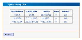
This section displays the core contents of the system routing table of the router.
