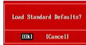
Pressing <OK> loads the default values that are factory settings for stable performance system operations.
