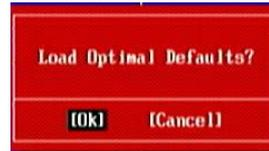
Pressing <OK> loads the default values that are factory settings for optimal performance system operations.
