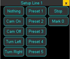
The Carousel controller provides up to three inputs that can be defined as shown. Once an input is defined, when it is "true" that function will be performed regardless of any other activity being commanded from the screen.
