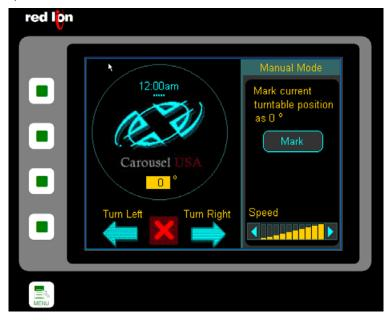
The speed graph in the lower right-hand corner of the screen adjusts the rotational speed during manual mode.
