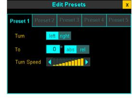
An absolute move of 30° will move the table 30° from the zero position. If multiple commands of this type are issued, no further action after the first will be seen as the turntable will already be at 30°.
