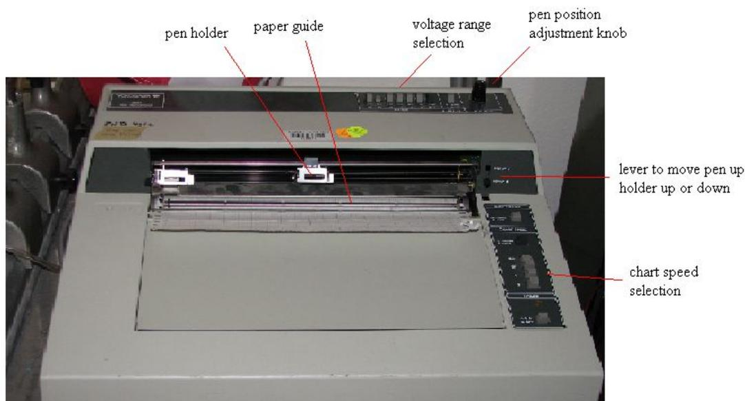
*Figure 3:* This is the strip-chart recorder that you will be using during the experiment. You can play around with the range and speed settings to see what works best.
