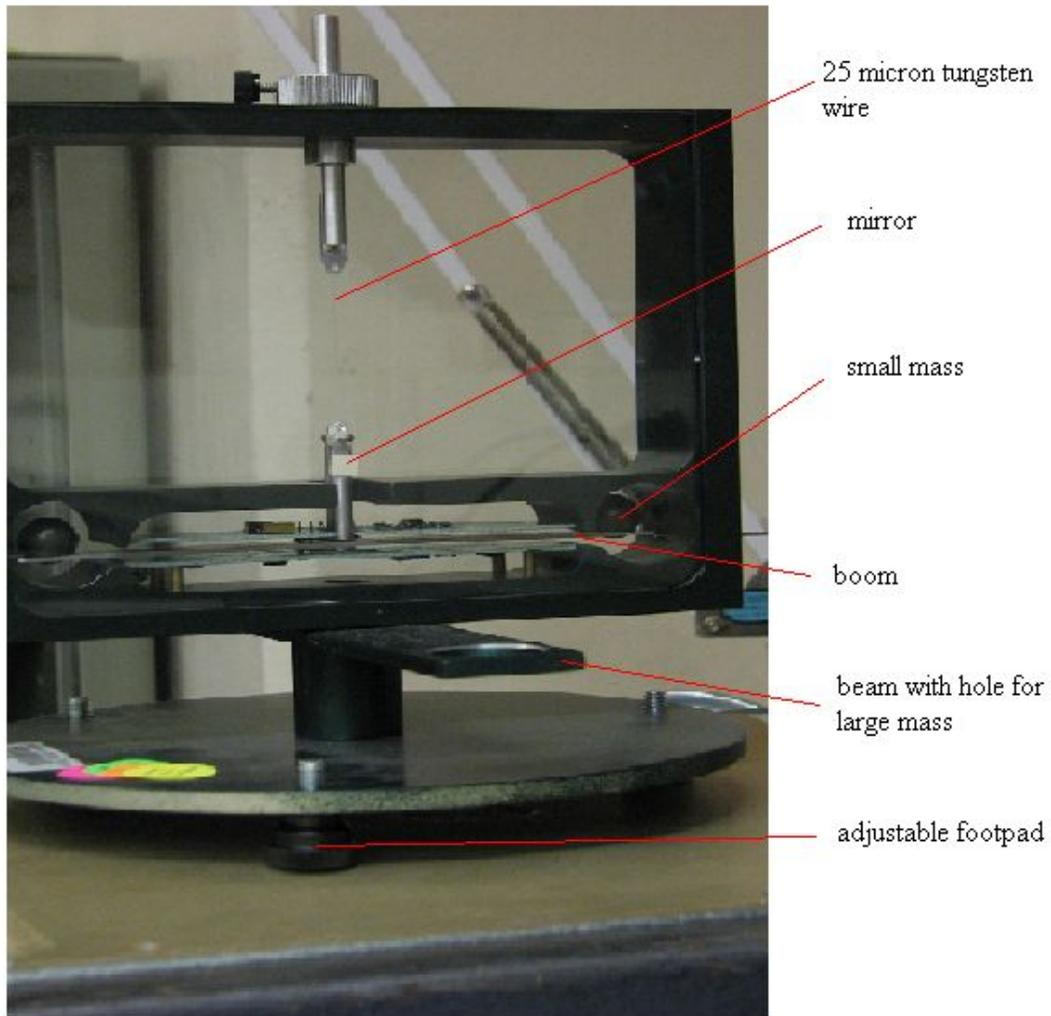
*Figure 2:* This labeled image of the Cavendish balance should be referred to while following the instructions in this manual.
