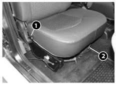
Seat backrest inclination adjustment lever
