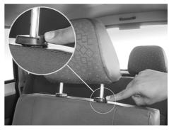
Release Button for Head rest height adjustment
