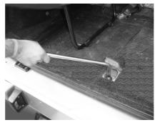
Loosening/Tightening of wheel winch screw
