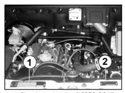
1. Chassis number plate (4SPTC-BS-III) 2. Body Shell (Cab) no. plate (4SPTC-BS-III)
