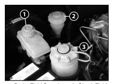
Brake Fluid Container 2. Clutch Fluid Container 3. Power Steering Container
