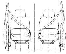
Seat-belt Arrangement on Driver & Co-driver's Seat
