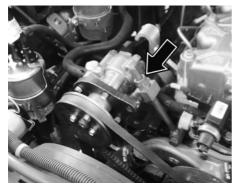
Power Steering Pump Belt Adjustment Nut
