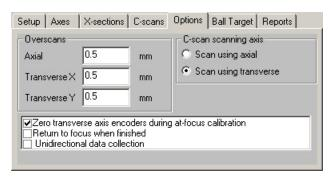
**Unidirectional data collection:** If your scanner has significant backlash, you may wish to specify unidirectional scanning to improve scan image quality, especially when performing fine resolution C-scans.
