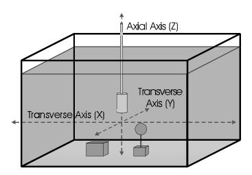
Depending upon the size and configuration of your tank, you may need to use different axis definitions. For example, if you are using a shallow tank, you may need to aim the transducer horizontally at the target, and name your axes accordingly.
