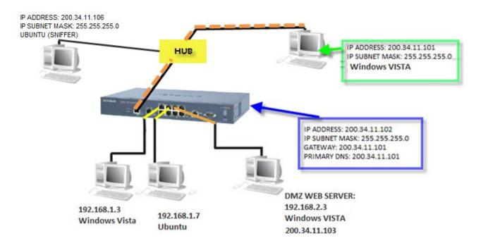
We setup VPN using on the external host "Netgear VPN client software". As far as the firewall concerns, the configuration is the following:
