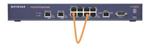
Then we connected also a PC to the switch and we execute a "ping" on the firewall interface. A great quantity of traffic started to run inside the loop so that the firewall immediately saturated and it was no more possible to accede to the configuration page.
