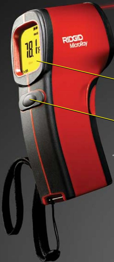
*Read smaller objects from farther away with a large, 15 to 1 Distance-to-Spot Ratio.*
