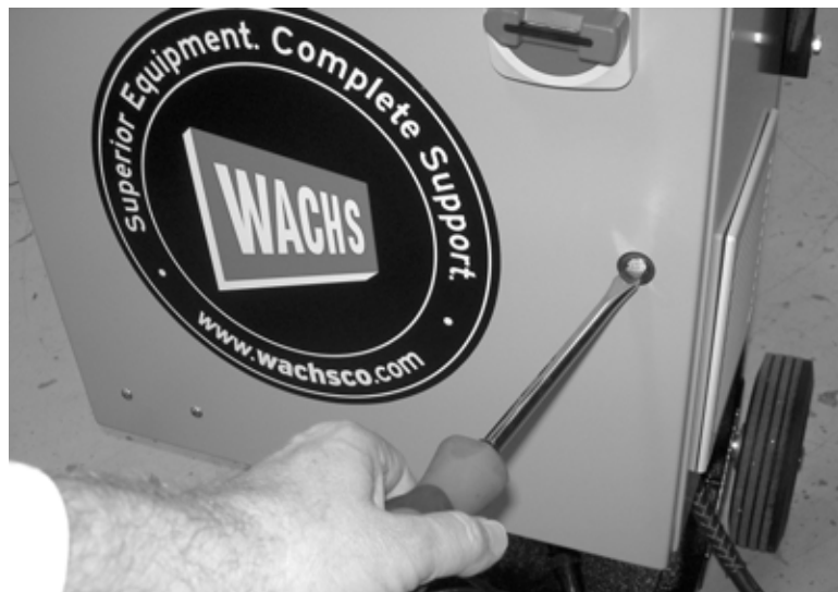
Figure 1-18. Loosen the screw before opening the cabinet door.
