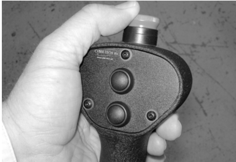
Figure 1-15. Push down the Emergency Stop button on the pendant to stop the machine and shut down power to the drive.
