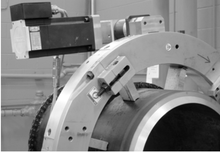
Figure 1-3. The SDE for LCSF machines is equipped with a right-angle adapter. The adapter mounts directly to the standard pinion assembly.
