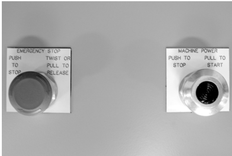
Figure 1-12. To enable the SDE, make sure the Emergency Stop button is pulled out, then pull the Machine Power button. The light in the center of the button will come on to indicate power is enabled.
